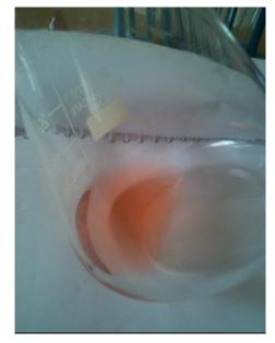
(c) IPE Figure 4: End Point Detection of S.A Vs S.B (HCl – Na<sub>2</sub>CO<sub>3</sub>)
