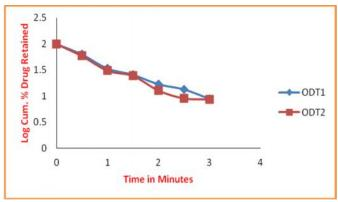
Fig 8: In vitro release curve of Thiabendazole tablet -First Order Release (ODT1 & ODT2)
