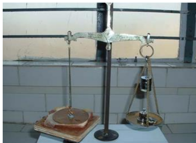
Fig-3: Fabricated bioadhesion testing instrument
