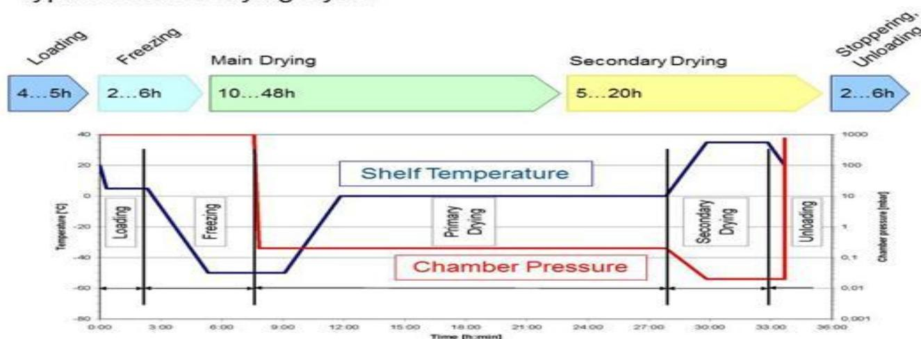
Fig. 1: Typical Freeze Drying Cycle
