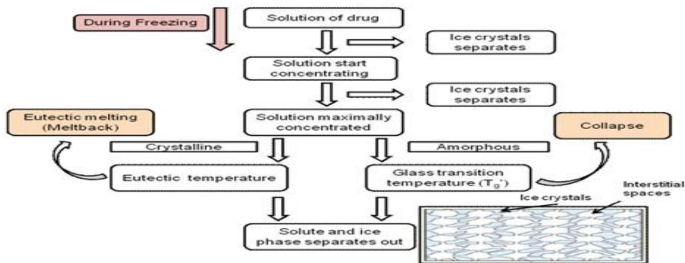
**Fig. 2:** Flowchart showing the concept of eutectic temperature and T<sub>g</sub> (glass Transition) and their importance during primary drying.
