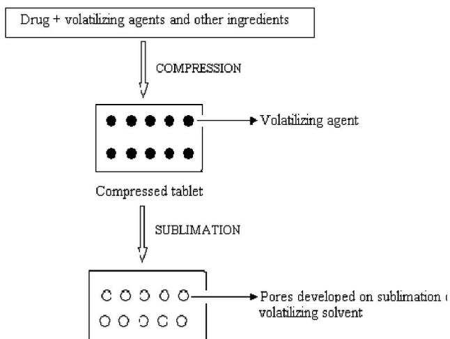
**Fig. 3:** Schematic Diagram of Sublimation Technique for Preparation of MDT
