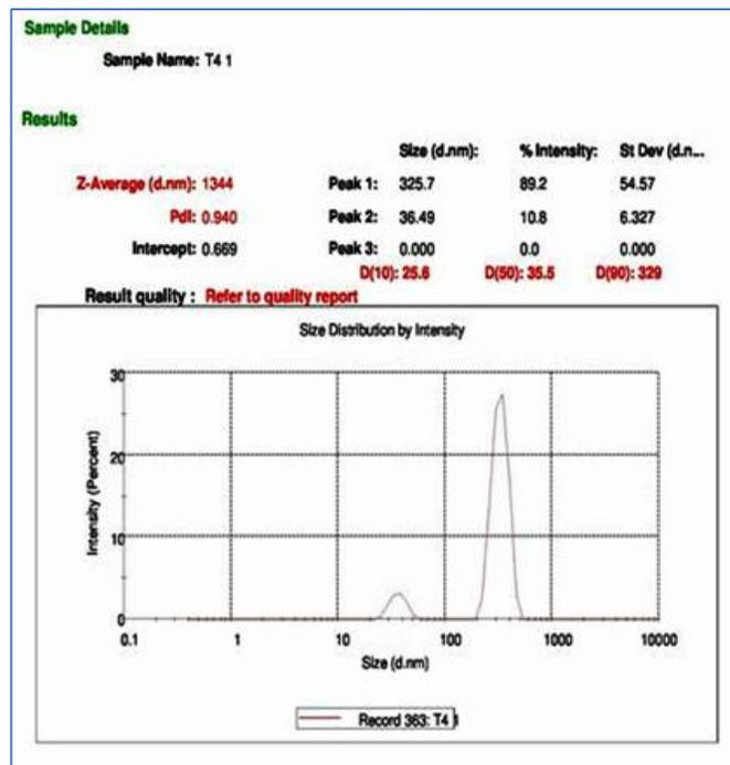
Figure 6: Droplet size and polydispersity determination by zetasizer
