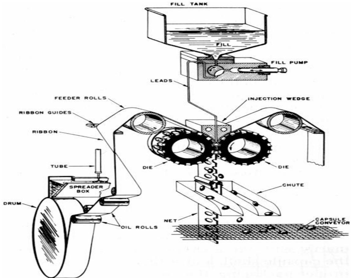
Figure 6: Schematic drawing of a rotary-die soft gelatin capsule filler (R.P. Scherer: Detroit, MI).
