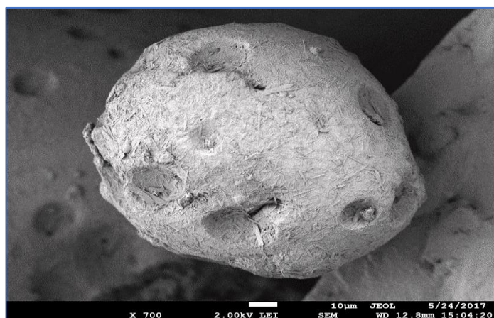
Fig. 9: Scanning Electron Photomicrograph of RM 6 Microsphere
